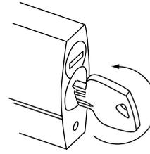
Insert control key and turn counterclockwise until stop is reached.
