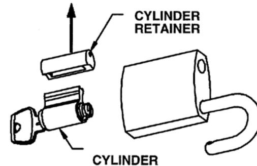
Remove cylinder retainer from cylinder for repining. Reverse steps to reassemble.
