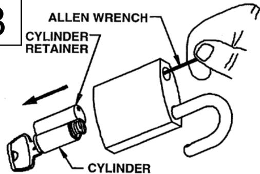
Insert a 5/64" Allen wrench and remove retainer screw as shown. Cylinder and retainer will drop out together.
