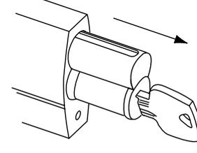
To remove key - return to vertical position and withdraw.
