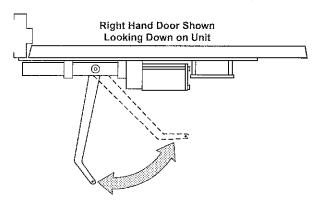
Remove arm and reinstall it on the spindle with the arm almost parallel to the frame face, before the spindle shaft can rotate far enough to create arm interference with the frame.
