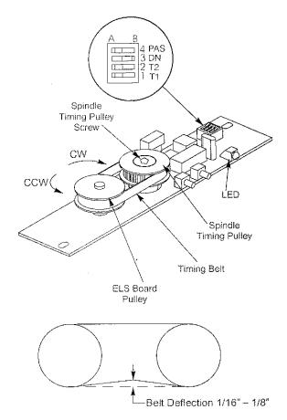
\*\*NOTE: If LED should turn off during the above procedure without any significant movement of ELS Board Pulley, this is not a problem. The timing zone range is large enough to allow for slight movement of ELS Board pulley during tightening of spindle timing screw.
